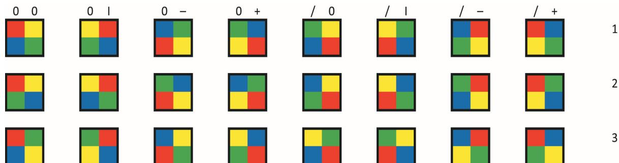
The figure above shows the simplified model of Poly-Universe. The categorization of elements in the rows is the following: if two elements are in two different rows, they cannot be moved onto each other using rotation or reflection. Elements in each row are transformed from the first element applying 1, 2 or 3 reflections.
